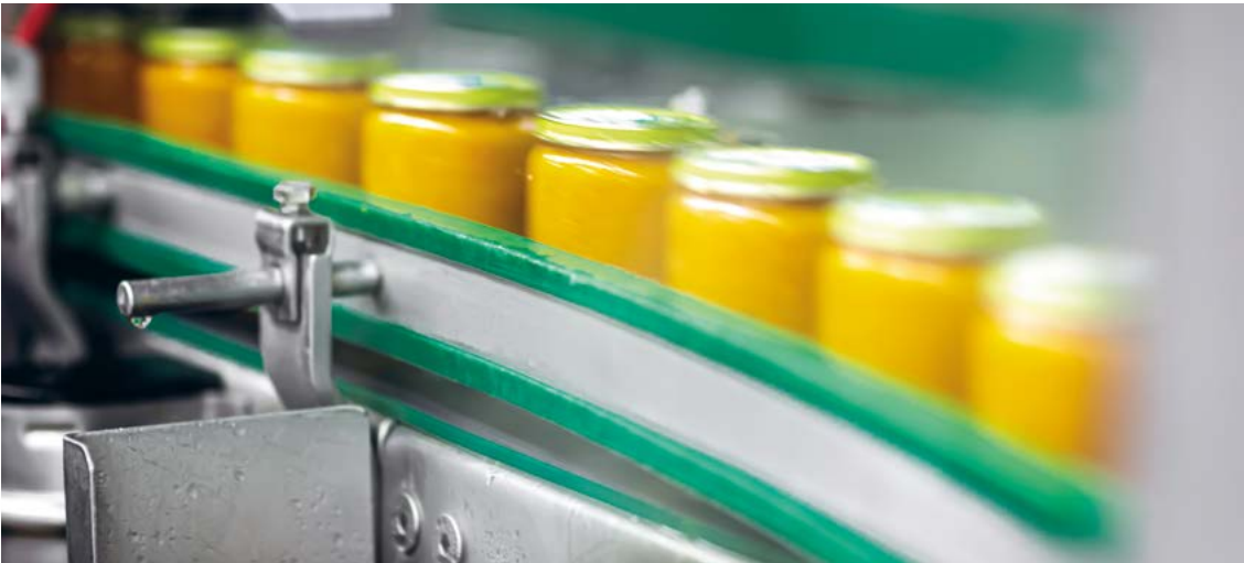
The glass used for HiPP jars is as thin as possible and as thick as necessary to remain intact during intensive production operations (see photo) and subsequent transport.
